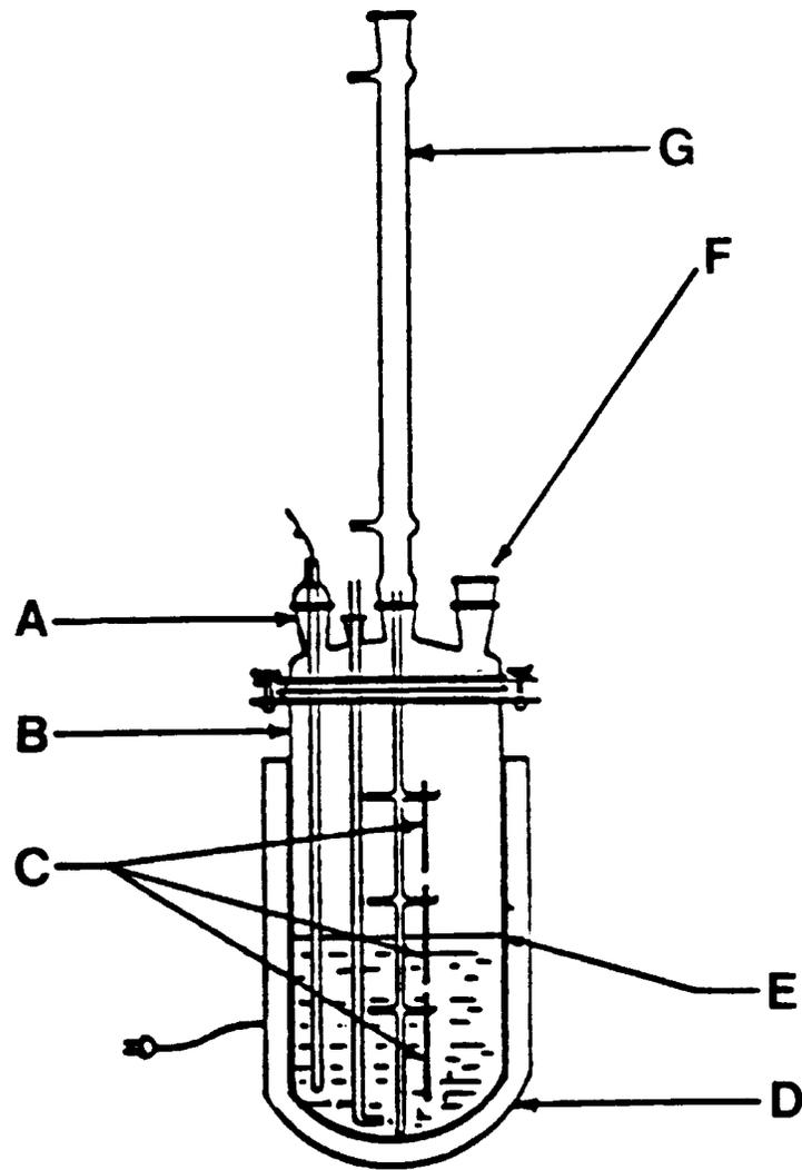
Figure 1. Typical resin flask that can be used as a versatile and convenient apparatus to conduct simple immersion tests. Configuration of the flask top is such that more sophisticated apparatus can be added as required by the specific test being conducted. A = thermowell, B = resin flask, C = specimens hung on supporting device, D = heating mantle, E = liquid interface, F = opening in flask for additional apparatus that may be required, and G = reflux condenser.
